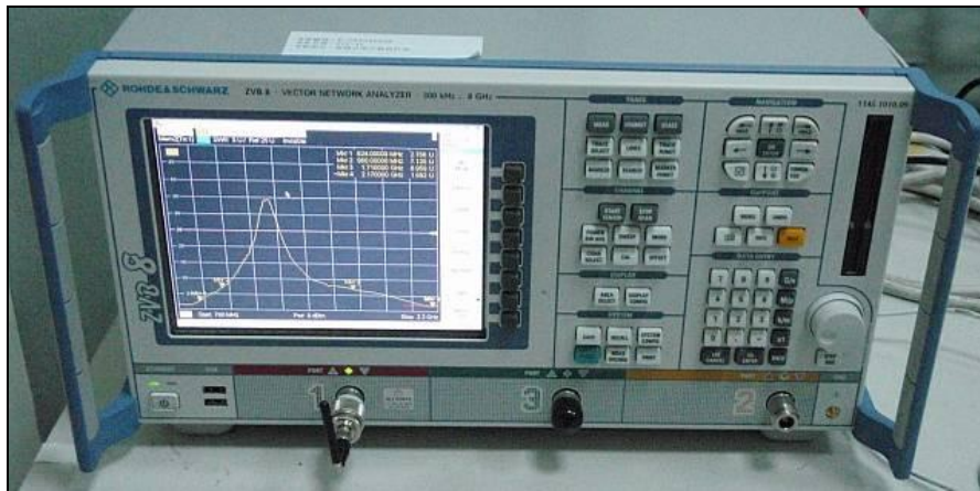
Figure 2 VNA for Return Loss and VSWR
