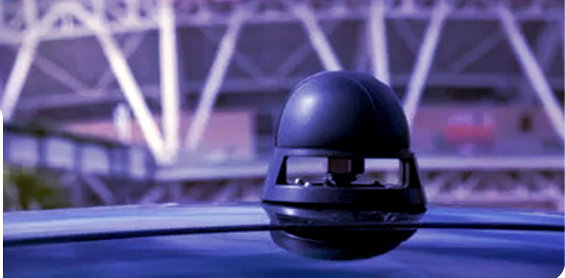
As for the Pantheon, "It's proven to hold up to all that very well," Dryden reports. It's also unobtrusive, he explains. "It's not one of those whip or fin antennas, where they stick up and can be vandalized. It's a smooth, dome-shaped antenna that can't break off or be damaged."
