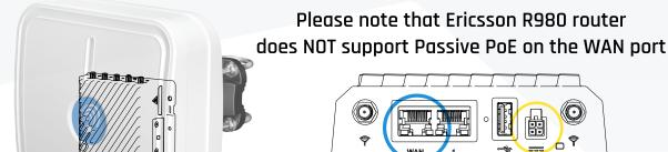
Before connecting PoE to your router, please check specification of your model. Connecting PoE to model that's not supporting PoE can damage your router.
