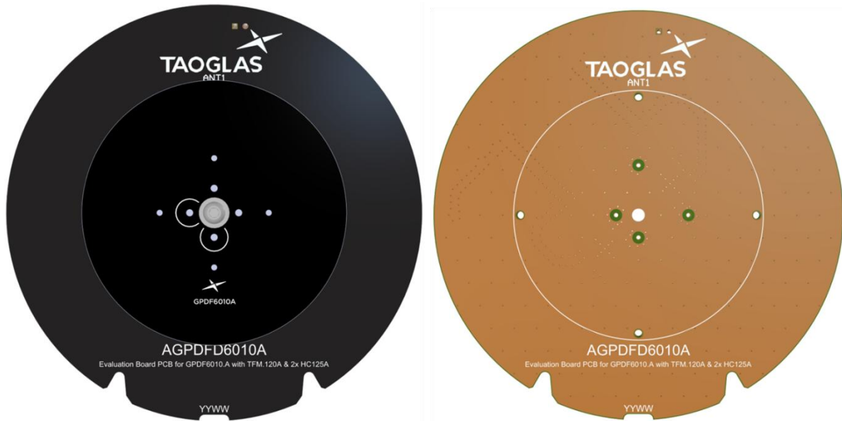
Top Side ( GPDF6010.A placement on 70x70mm PCB)
