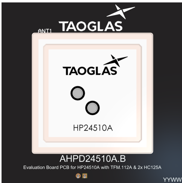
Top Side ( HP24510A placement on 70x70mm PCB)
