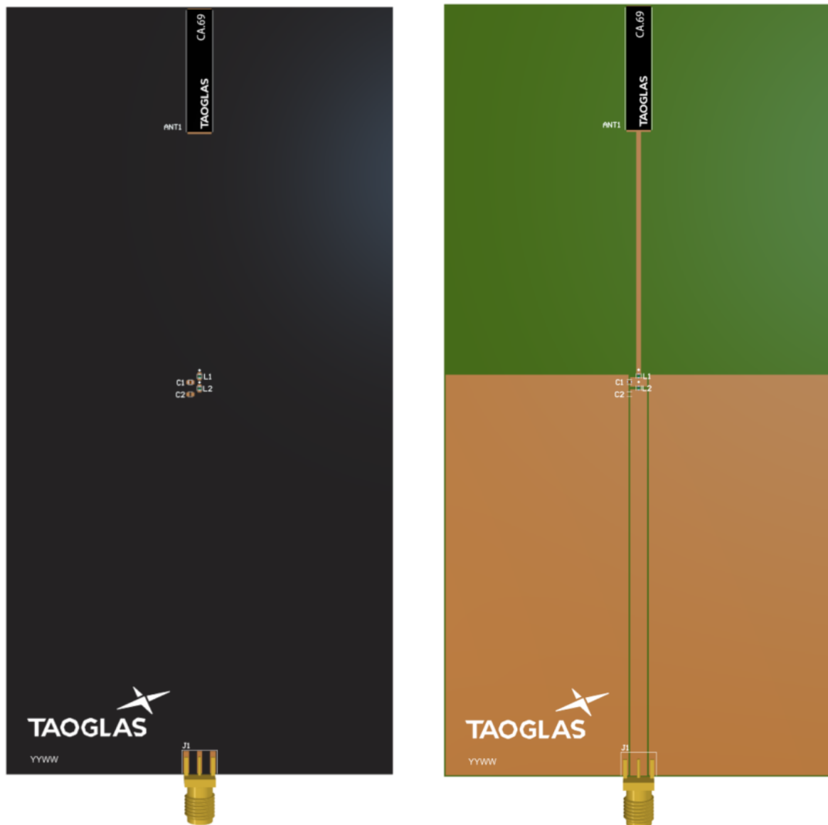
Top Side (CA.69 placement on 159.5x80mm PCB)
