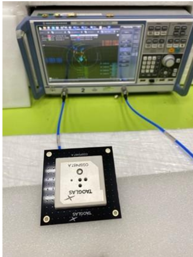
VNA Test Setup
