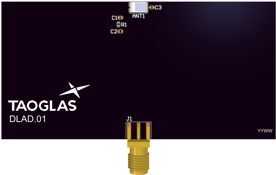
Above is a 3D model of the DLA.01 on a PCB.
