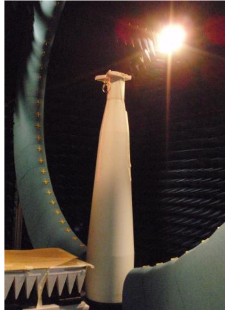
Free space antenna setup and Satimo SG64 3D-chamber.
