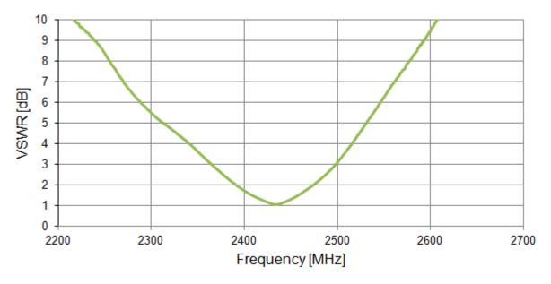
Figure 3. VSWR of the FXP75 antenna from 2200 MHz to 2700 MHz.
