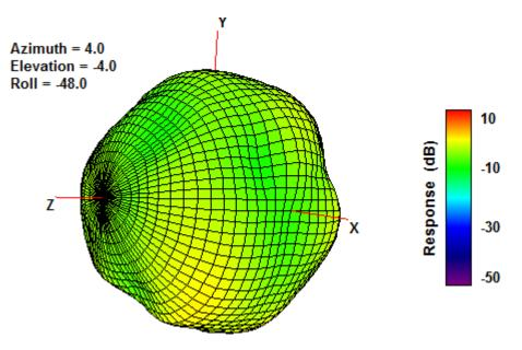
Figure 7. 3D Radiation Pattern at 2450 of the FXP75 Antenna.
