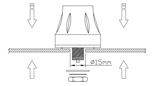
**Recommended torque for mounting: 5-7Nm** (Torque value obtained with antenna mounted on 1mm thick SUS-316 bracket)
