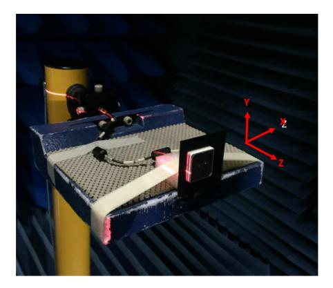
Tested on a 70\*70mm ground plane.
