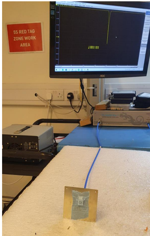
VNA Test Setup on a 50x50mm Ground Plane
