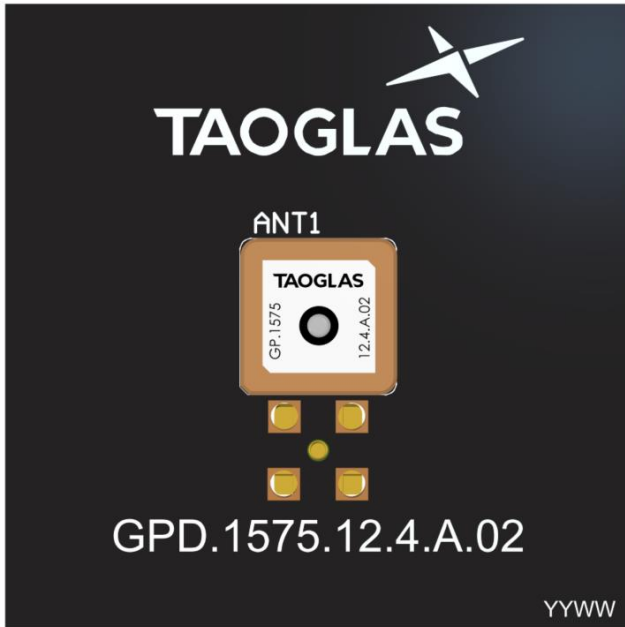
Top Side (GP.1575.12.4.A.02 placement on 50x50mm PCB)
