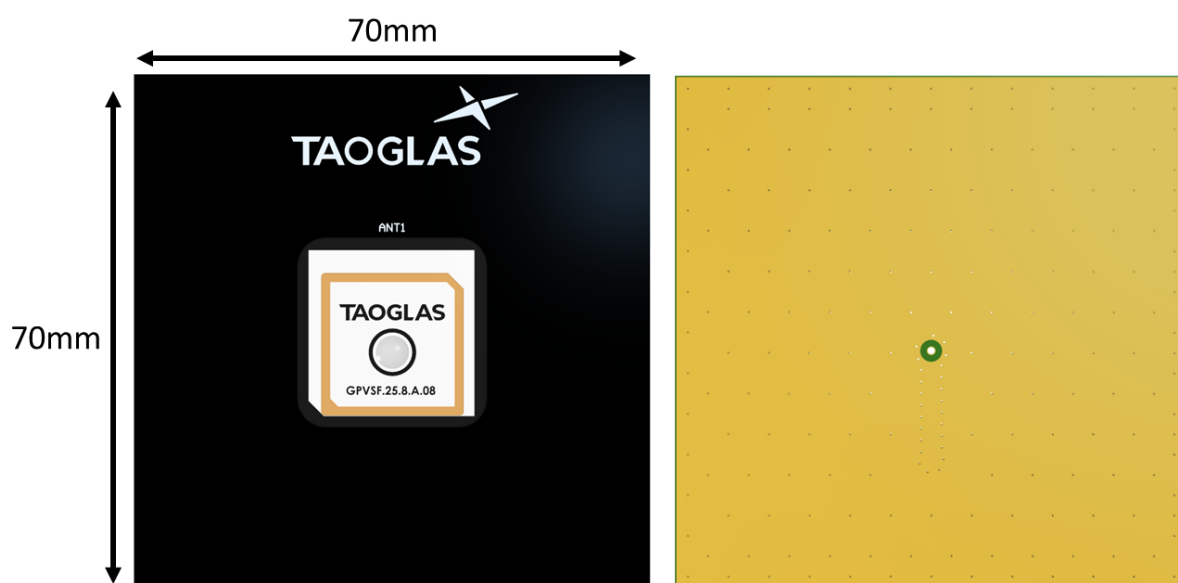
Top Side (70x70mm example PCB Reference Design)
