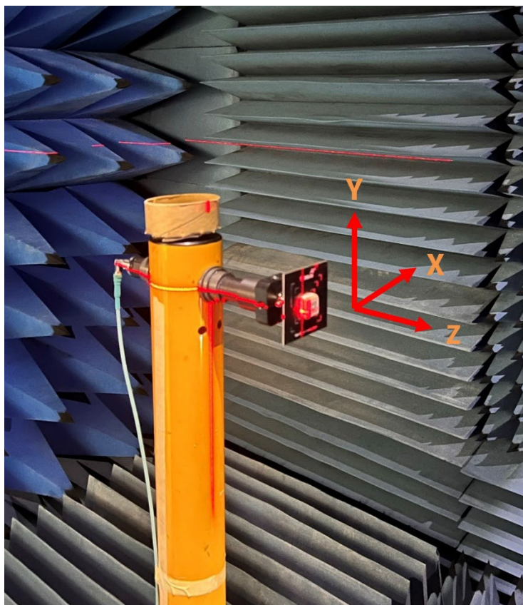
Chamber Test Set-up
