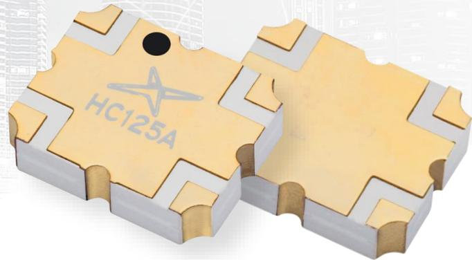
The Taoglas HC125A is a low profile, high performance, 3dB hybrid coupler in an easy to integrate surface mount package. It is designed for multi feed GNSS applications. The HC125A is particularly used for applications where balanced power and low noise amplifiers are required. It has low insertion loss and tight amplitude and can be used in power applications up to 30 Watts. It has been engineered to cover the full GNSS bandwidth of 1150 – 1630MHz.
