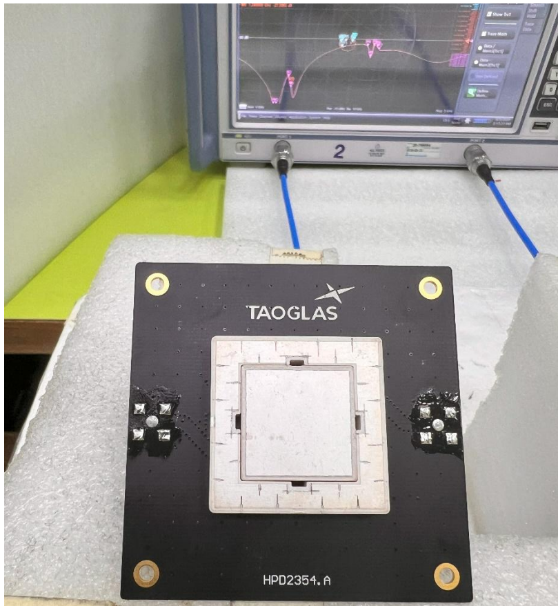
VNA Test Set-up
