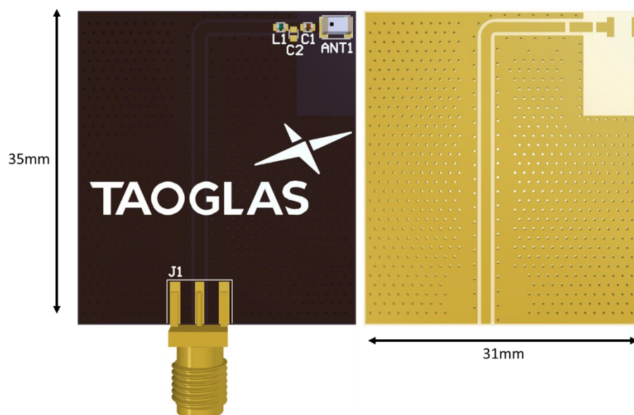
Top Side (ILA.68 placement on 35x31mm PCB reference design)
