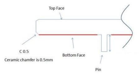
Red Line shows the adhesive without Liner – thickness 0.08~0.1mm
