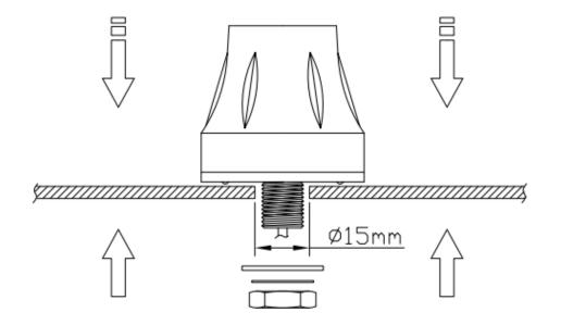
Recommended torque for mounting is 2.94 N·m Maximum torque for mounting is 3.92 N·m
