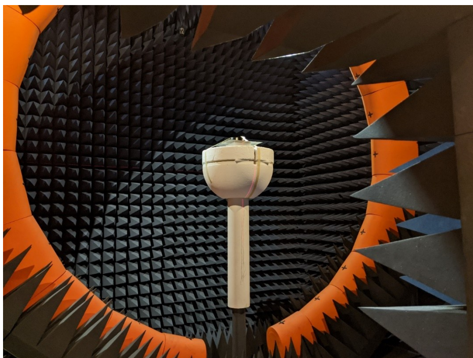
Antenna tested with underside-notch/logo centered along Y-Axis.
