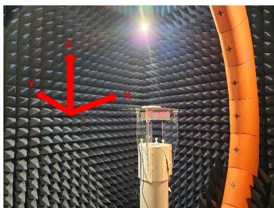
Set-up on a 30x30cm Ground Plane
