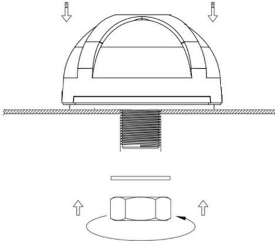
**Recommended torque for mounting: 5-7Nm**
