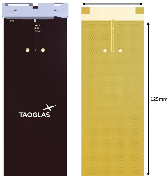
Top Side (MPA.66.A placement on 50x50mm PCB)
