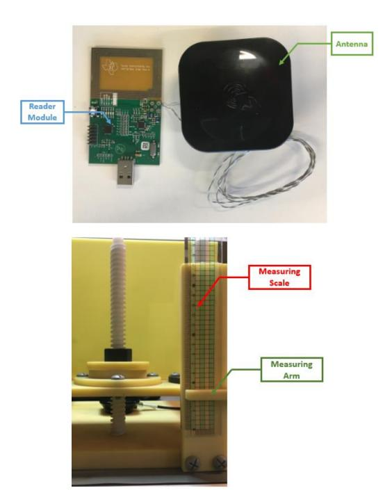
The test sample is placed on a thin sheet of plastic connected to the moveable part of the fixture. Then the distance is carefully adjusted until the reader can no longer read the sample, thus the maximum interrogation distance is displayed in the ruler.
