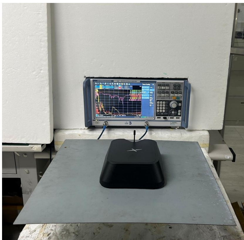
VNA Test Set-up on a 30x30cm Metal Ground Plane with 30cm cables.
