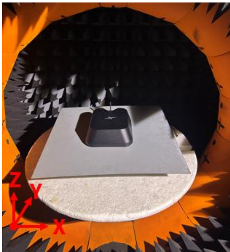
Chamber Test Set-up on a 30x30cm Metal Ground Plane with 30cm cables.
