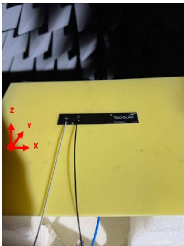
Chamber Test Setup on 2mm ABS
