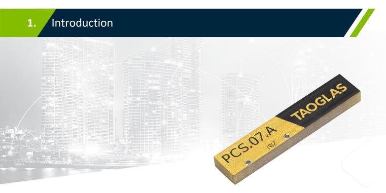
The PCS.07.A is a low profile SMT cellular antenna designed for direct SMT mount on the device PCB. It provides highest efficiency in very small factor 35\*7\*3mm. It is more resistant to detuning compared to other antenna integrations. If tuning is required it can be tuned for the device environment, while there is no need for new tooling. Its rectangular shape and very small size makes it very easy to integrate – can be mounted directly on the edge of the PCB board.
