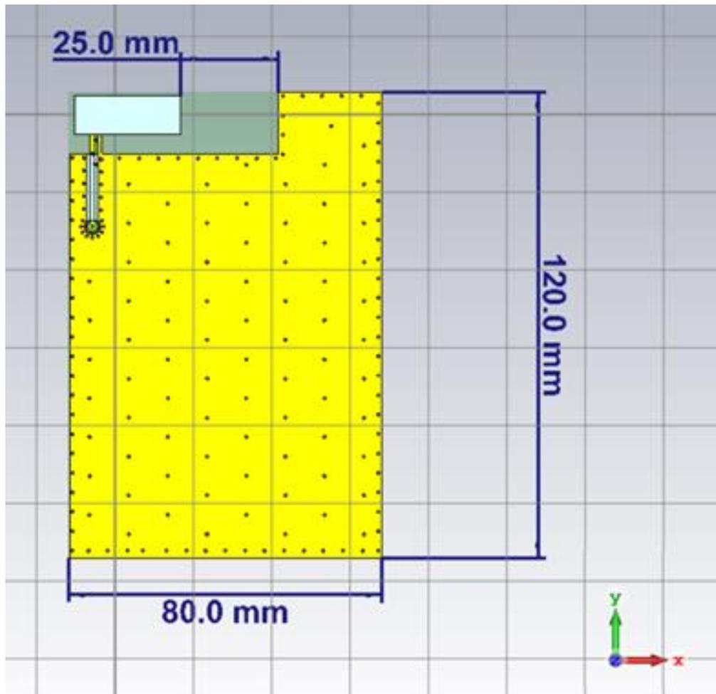
For minimal (0.2 dB) performance impact, a clearance of 25mm is recommended. Return loss and efficiency 25, 35 and 50mm clearance are shown below:
