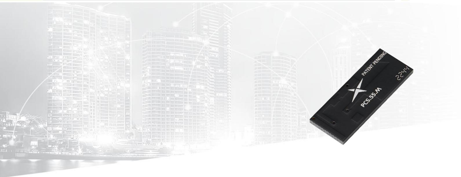
The PCS.55.M, is a patent pending compact cellular antenna designed specifically for IoT devices with small ground planes. It combines revolutionary antenna design techniques with the antenna integration experience of Taoglas to provide a solution for wideband coverage of both 5G/4G LTE and GNSS bands, including the most challenging 600-700MHz bands.
