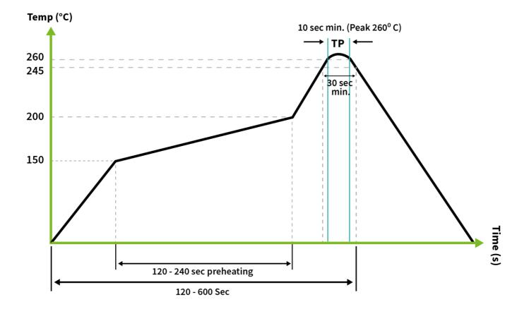
The RECE.20279.001E.01 can be assembled by following the recommended soldering temperatures are as follows:
