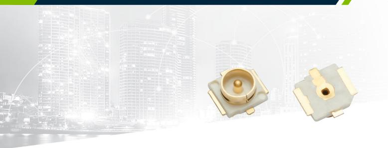
Part of the Taoglas SMD Mount Receptacle, the RECE.20279.001E.01 is a 3-pad type wire-to-board SMD receptacle that is ultra-small, lightweight and low profile, 2.5mm max. With an operational frequency range of DC to 8 GHz the RECE.20279.001E.01 is gold plated to provide superior performance and allow for ease of mounting with the male RF connector.
