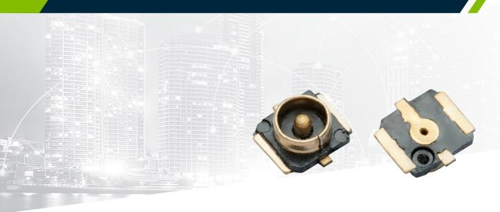
Part of the Taoglas SMD Mount Receptacle the RECE.20369.001E.01 is a 3-pad type wire-to-board SMD Receptacle solution that is ultra-small, lightweight and low profile (1.6mm MAX.) with an operational frequency range of DC to 8 GHz. Taoglas the RECE.20369.001E.01 is gold plated to have superior performance and allow easy mounting of the male RF connector.
