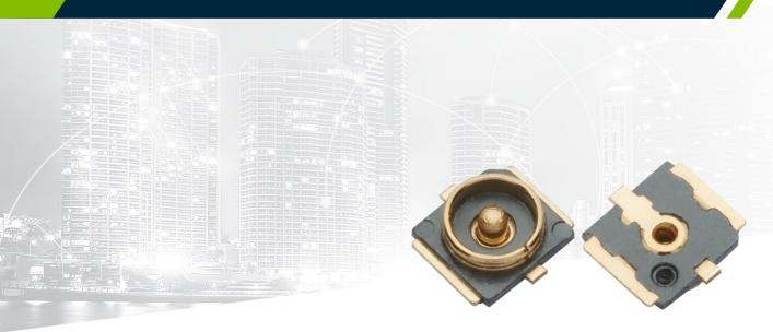
Part of the Taoglas SMD Mount Receptacle, the RECE.20449.001E.01 is a 3-pad type wire-to-board SMD Receptacle solution that is ultra-small, lightweight, and low profile, 1.6mm max. with an operational frequency range of DC to 8 GHz the RECE.20449.001E.01 is gold plated to provide superior performance and allow easy mounting of the male RF connector.
