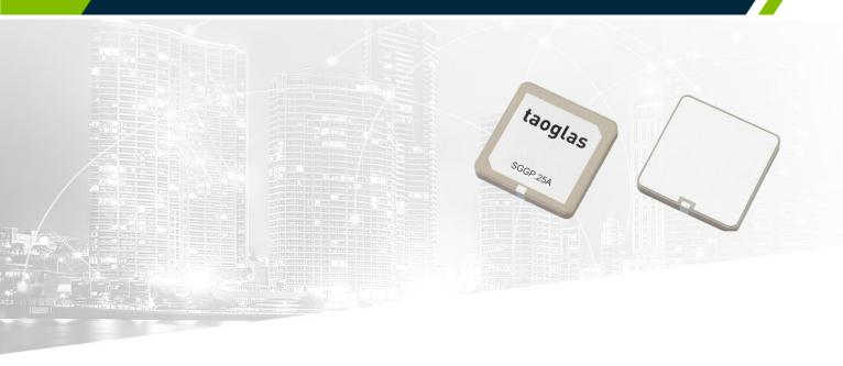
The Taoglas SGGP.25 is a ceramic GPS/GLONASS/Galileo passive patch antenna designed for optimal performance on GPS L1/Galileo E1 band (1575.42 MHz) and GLONASS L1 band (1602 MHz). With a low-profile thickness of just 4mm and convenient mounting via standard SMD process, it is ideal for high-volume, low-cost assembly applications.
