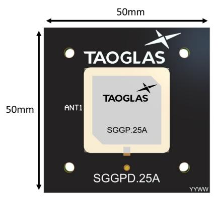
Top Side (SGGP.25.4.A.02 placement on 50x50mm ground plane)
