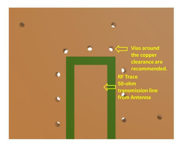
Top view of the PCB, showing transmission lines and integration notes.  $\label{eq:pcb}$
