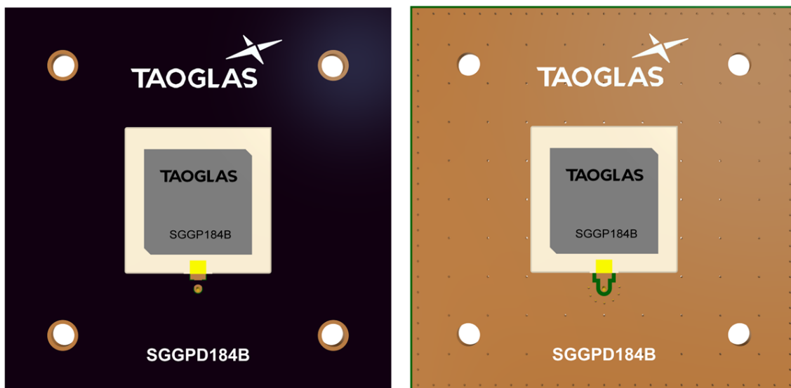
Top Side (SGGP184B placement on 50x50mm PCB reference design)
