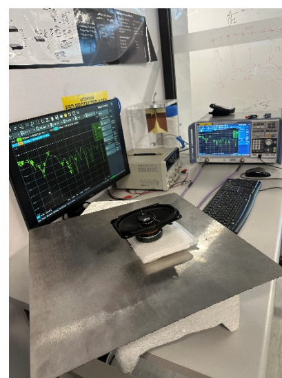
60 x 60cm Ground Plane With 1in Foam Spacer
