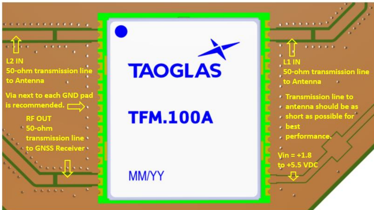
TFM.100A module mounted on a PCB, showing transmission lines and integration notes.
