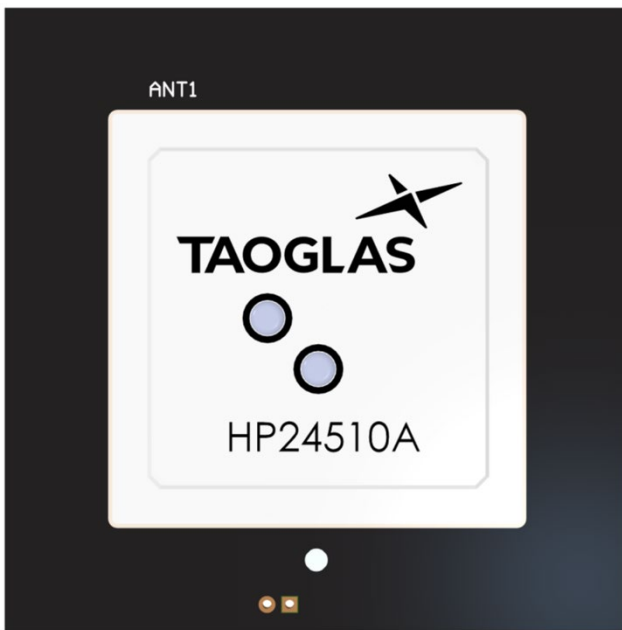
Top Side ( HP24510A placement on 70x70mm PCB)
