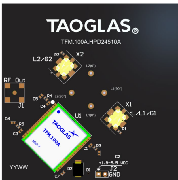
Top Side ( HP24510A placement on 70x70mm PCB)
