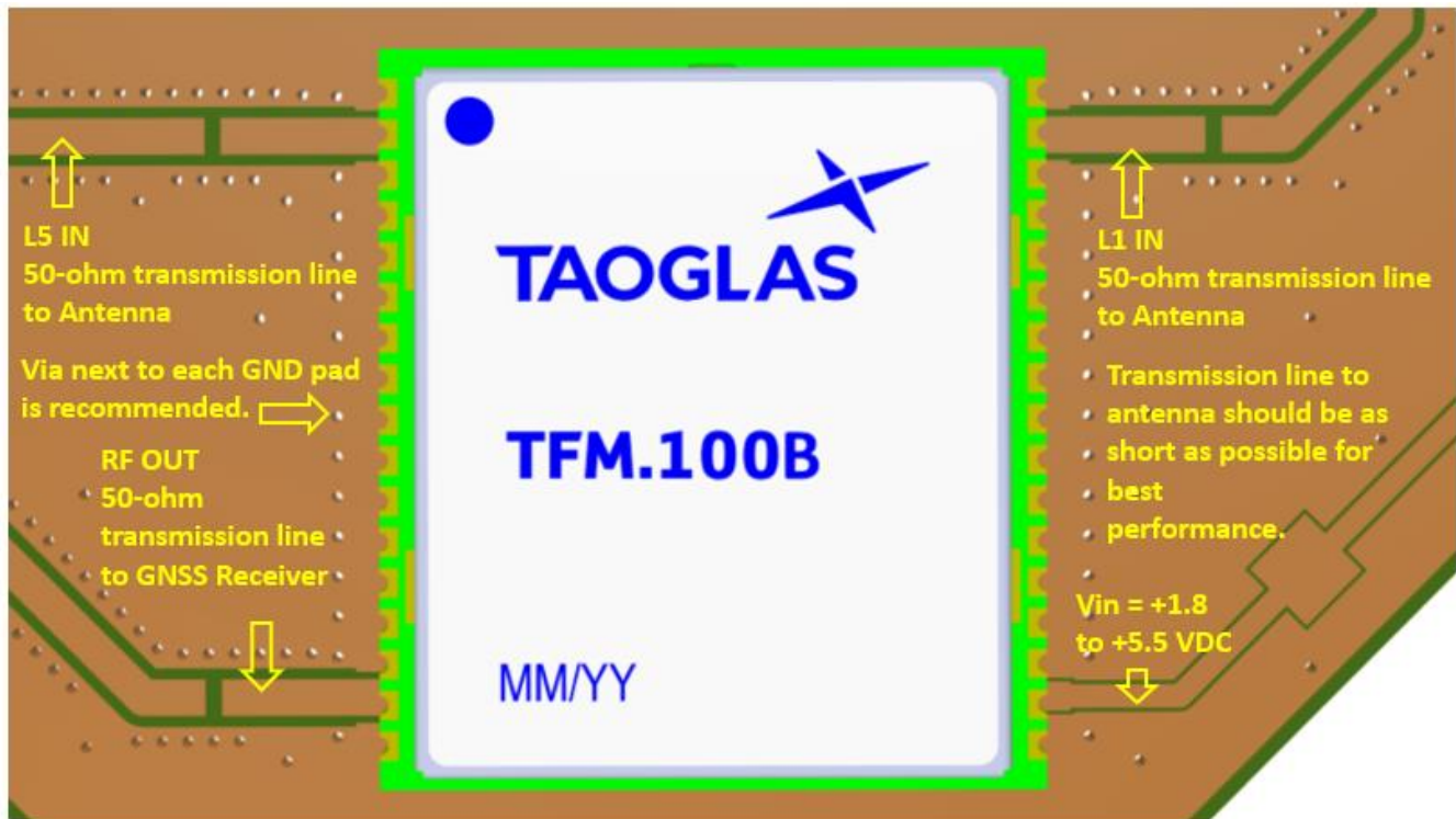
TFM.100B module mounted on a PCB, showing transmission lines and integration notes.
