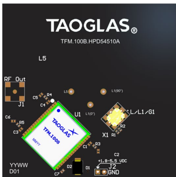
Bottom side (TFM.100B placement including HC125A )
