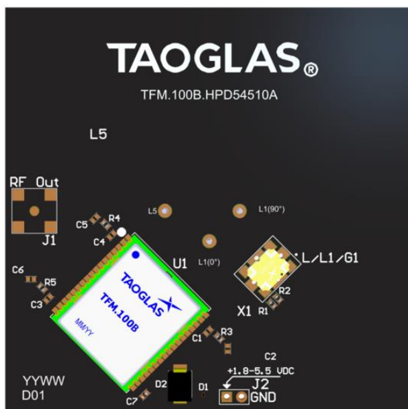
Bottom side (TFM.100B placement including HC125A )
