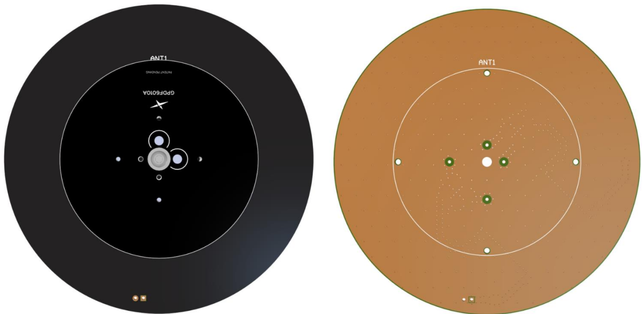
Top Side (GPDF6010.A Placement on Ø100mm PCB)
