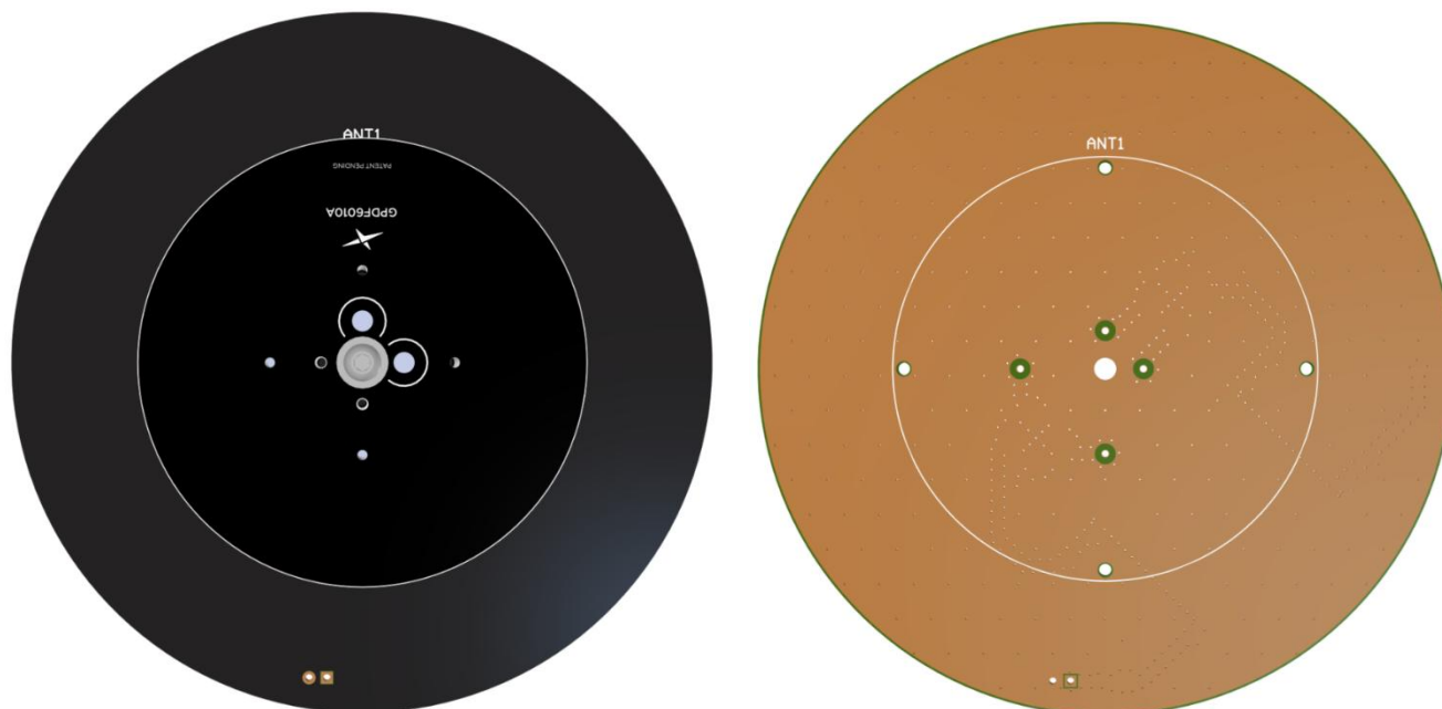
Top Side (GPDF6010.A Placement on Ø100mm PCB)
