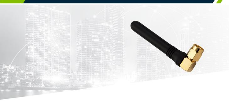
The Taoglas TI.08.C.0112 is a high performance antenna covering both 915MHz and 868MHz, small form factor, dipole omni-direction terminal mount antenna. This antenna features an SMA(M) right angle connector as standard.
