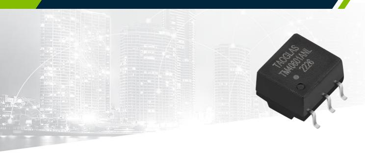
Featuring a compatible footprint with industry BMS Transformers, and designed to work in demanding automotive environmental conditions, the Taoglas TM40601ANL is a BMS Transformer with Common Mode Choke of 12 pins and Dual channel for Operation voltage of 1500VDC.
