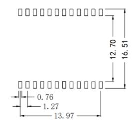
$\label{eq:Suggested} Suggested \ pad \ layout$  Dimensions are in millimeters with the following tolerances: X.XX =  $\pm 0.10$
