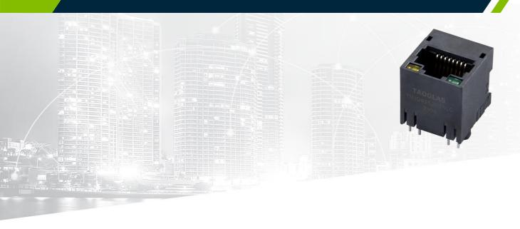
Featuring a popular footprint and compatible package to industry RJ45 Integrated Connectors standards, the Taoglas TMJD4152NENLC is an RJ45 Integrated Connector 10/100 Base-T Vertical with Unshielded body design and with PoE technology of 350mA.
