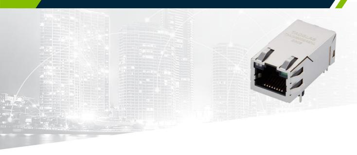
Featuring a popular footprint and compatible package to industry RJ45 Integrated Connectors standards, the Taoglas TMJM6002A9NL is an RJ45 Integrated Connector 2.5G Base-T Single Port Tab-UP with shielded EMI Finger and Long Body design that offers space for PoE++ (720mA) capabilities.
