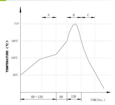
A.Preheating B.Soldering C.Gradual Cooling Tip temperature:260±5°C.
