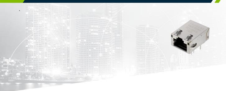
Featuring a popular footprint and compatible package to industry RJ45 Integrated Connectors standards, the Taoglas TMJUTGW0021103425 is an RJ45 Integrated Connector 1G Base-T Single Port Tab Up with shielded EMI Finger and Low-Profile design for extra space.
