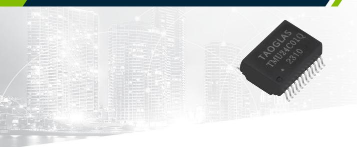
Featuring a compatible footprint with industry LAN transformers, and designed to work in demanding industrial environmental conditions, the Taoglas TMU24C01Q is a 2.5G Base-T Single Port of 24pin with Transformer and Common Mode Choke designed for PoE++ (720mA) capabilities.
