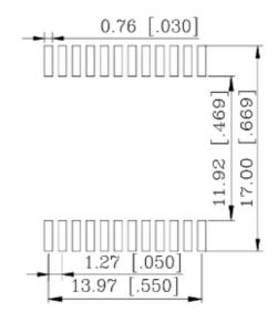
Suggested pad layout Dimensions are in millimeters with the following tolerances:  $X.XX = \pm 0.10$
