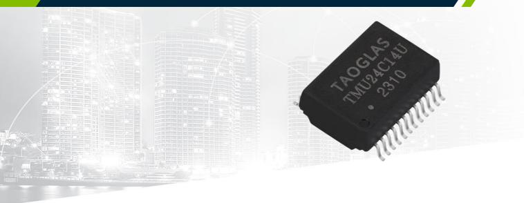
Featuring a compatible footprint with industry LAN transformers, and designed to work in demanding industrial environmental conditions, the Taoglas TMU24C14U is a 1G Base-T Single Port of 24pin with 3Wire and Transformer which makes it suitable for PoE Ultra (1100mA) applications in Industrial environments.
