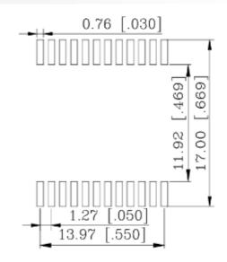
$\label{eq:Suggested} Suggested \ pad \ layout$  Dimensions are in millimeters with the following tolerances: X.XX =  $\pm 0.10$
