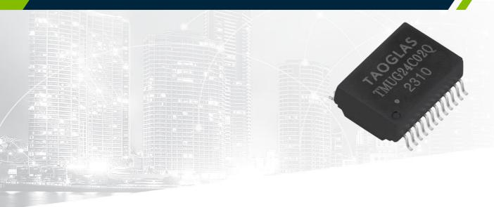
Featuring a compatible footprint with industry LAN transformers, and designed to work in demanding industrial environmental conditions, the Taoglas TMUG24C02Q is a 10G Base-T Single Port of 24pin with Transformer and Common Mode Choke which makes it suitable for PoE+ (720mA) applications in Industrial environments.
