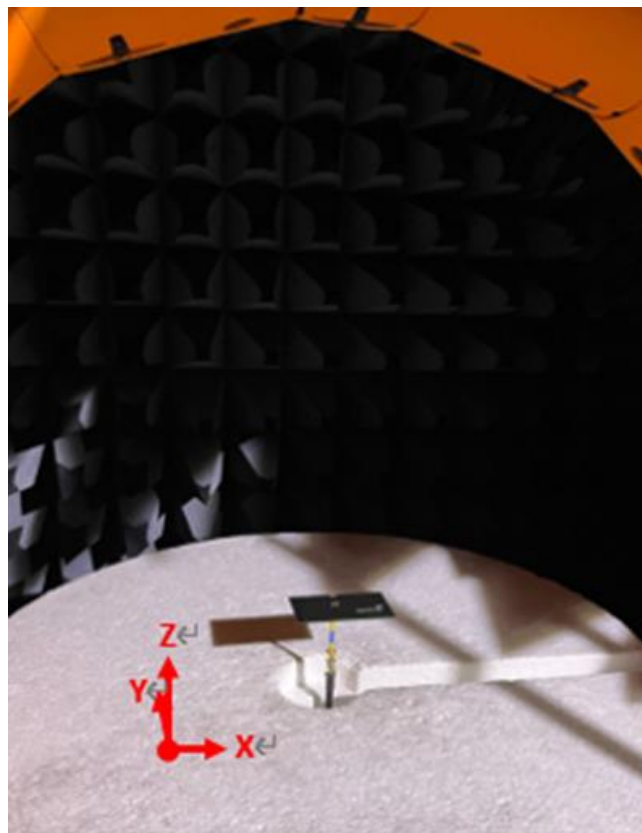
Chamber test setup on a 90x50mm Evaluation Board
