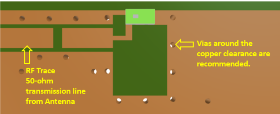
WLA.04 antenna mounted on a PCB, showing transmission line and integration notes.
