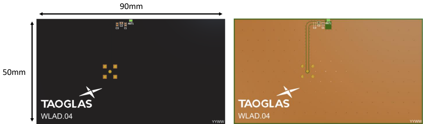
Top Side (WLA.04 placement on 90x50mm PCB)
