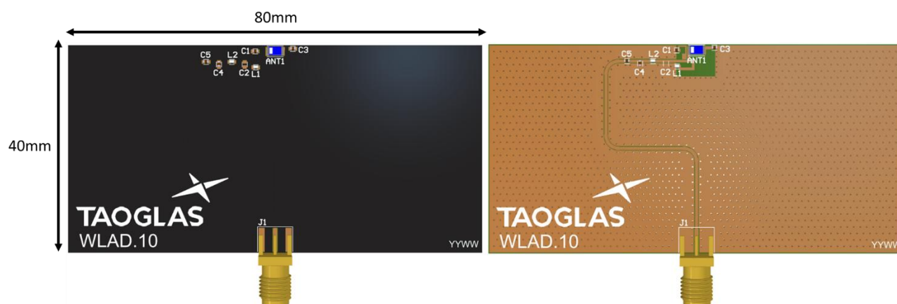
Top Side (WLA.10 placement on 80x40mm PCB)
