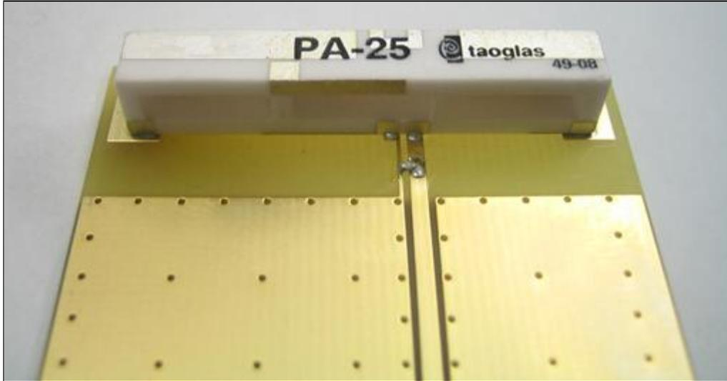
**Figure 18.** Antenna location on EVB (front view)..
